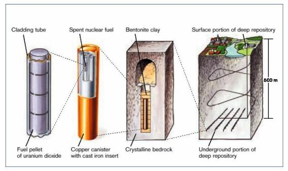
Multiple barriers prevent the radionuclides from reaching the ground surface. Source: Guais (2003).
