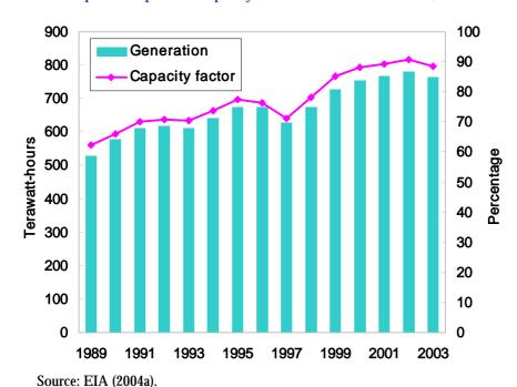
Figure 8 Nuclear plant output and capacity factor in the United States, 1989-2003
