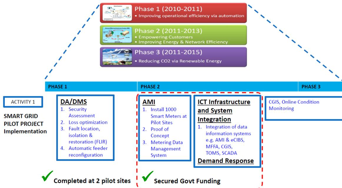
Notes: AMI – Advanced Metering Infrastructure, eCIBS – e-Customer Information & Billing System, MFFA – Mobile Field Force Automation, CGIS – Corp Geospatial Information System, TOMS – Transmission Outage Mgmt System, SCADA – Supervisory Control and Data Acquisition 23
