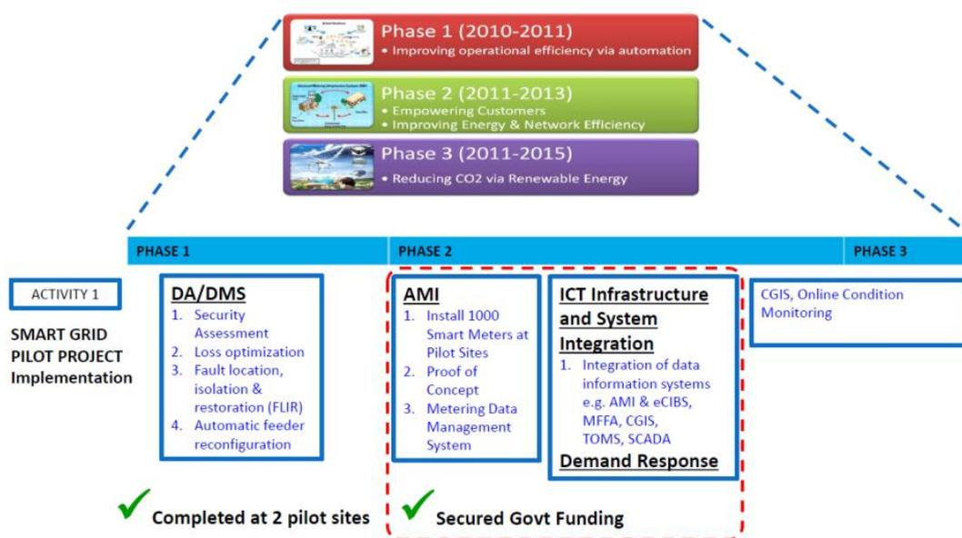
Notes: AMI – Advanced Metering Infrastructure, eCIBS – e-Customer Information & Billing System, MFFA – Mobile Field Force Automation, CGIS – Corp Geospatial Information System, TOMS – Transmission Outage Mgmt System, SCADA – Supervisory Control and Data Acquisition
