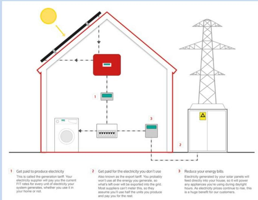
Figure 7-8: Net-metering mechanism<sup>111</sup>
