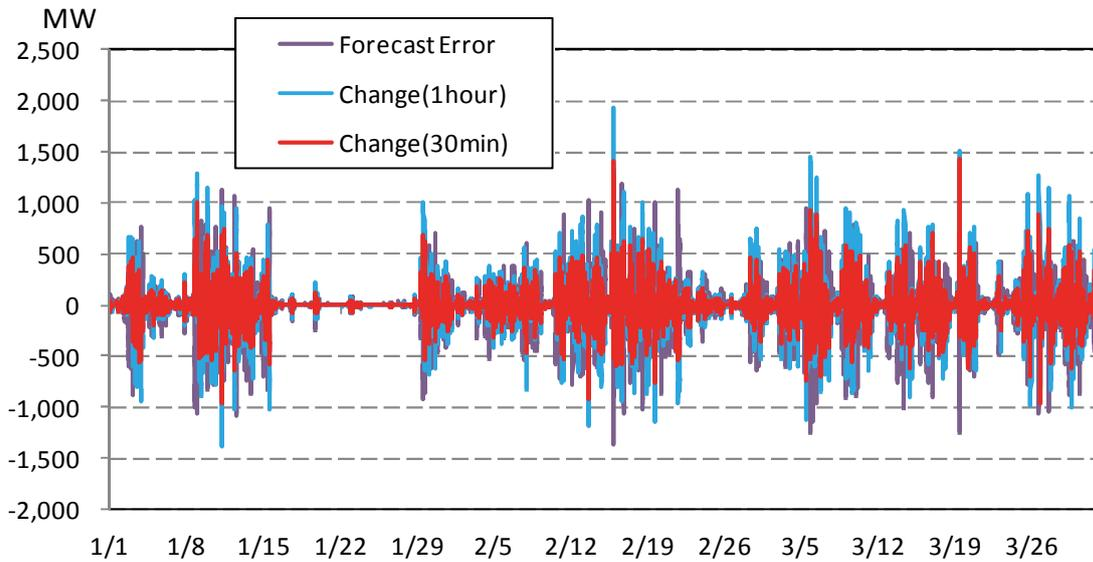
**Figure 4-11 Forecast Errors of Output of Wind Generation and Output Changes by Unit Time**
