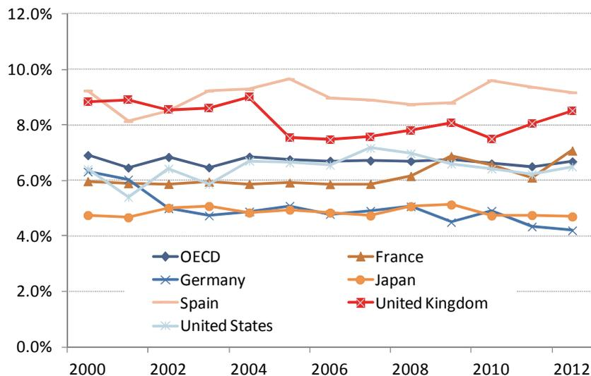
**Figure 3-3 Comparison of Transmission and Distribution Loss Rates**
