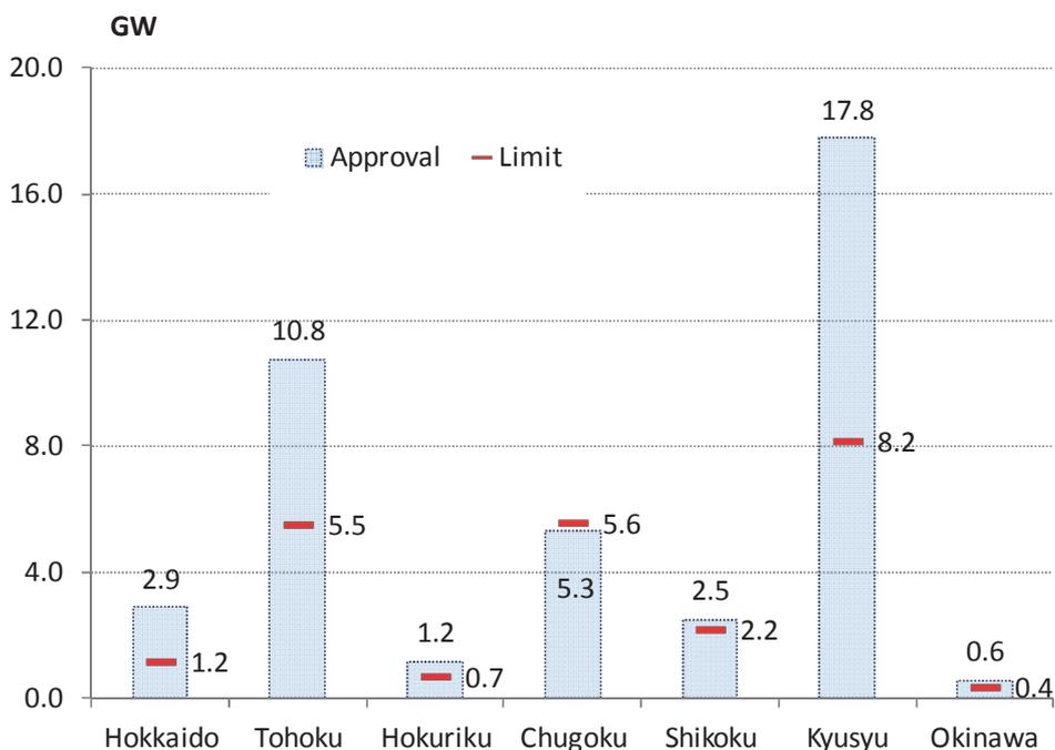
**Figure 3-7 Acceptable Limit of Power by PV Generation and Amount Approved under the FIT System**
