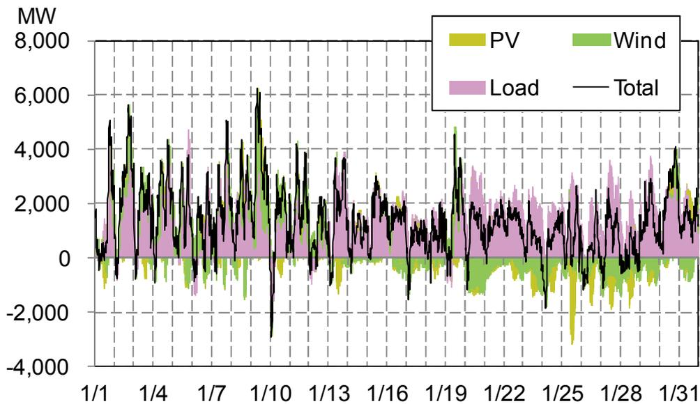
**Figure 4-8 Forecast Errors of Load, Output of Wind Generation and Output of PV Generation**
