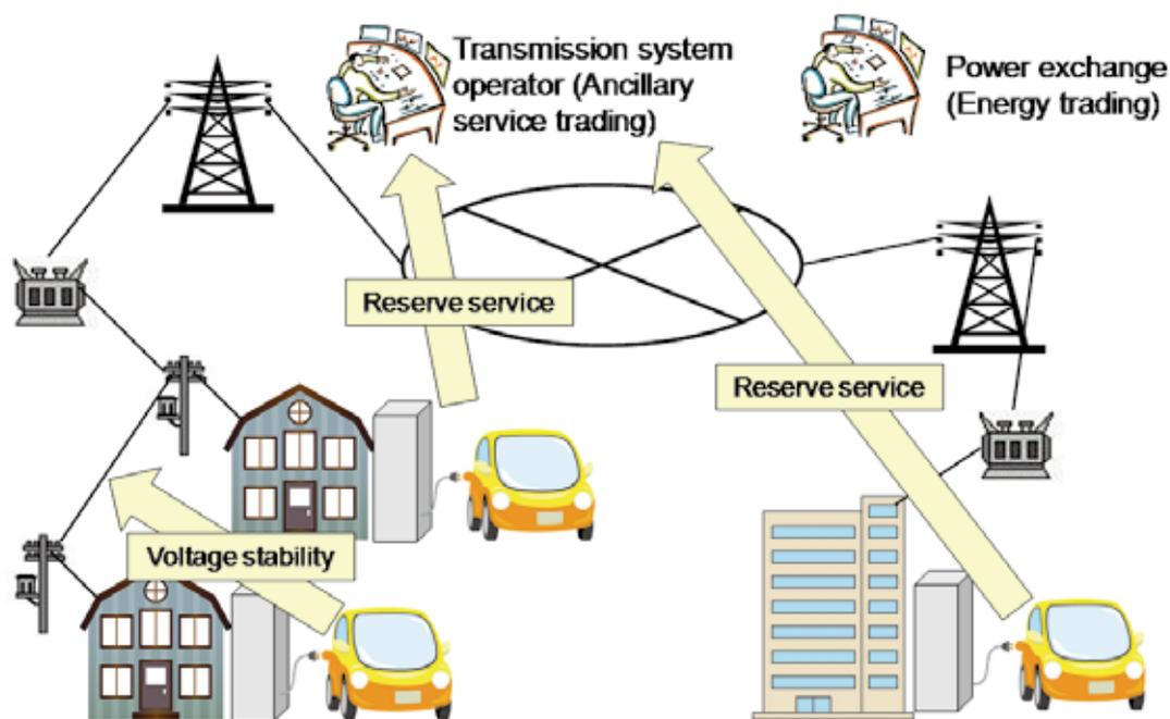
**Figure 4-16 Concept of Grid Integration of EVs**
