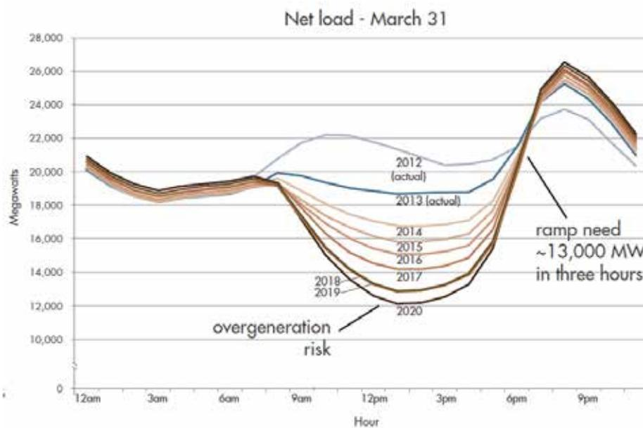
**Figure 3-6 The Duck Curve Shows Steep Ramping Needs and Overgeneration Risk**
