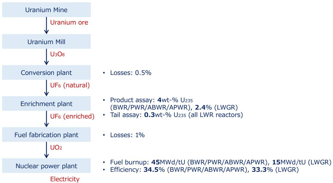
Figure 35 Front-end model for the fuel cycle (take LWR for example)
