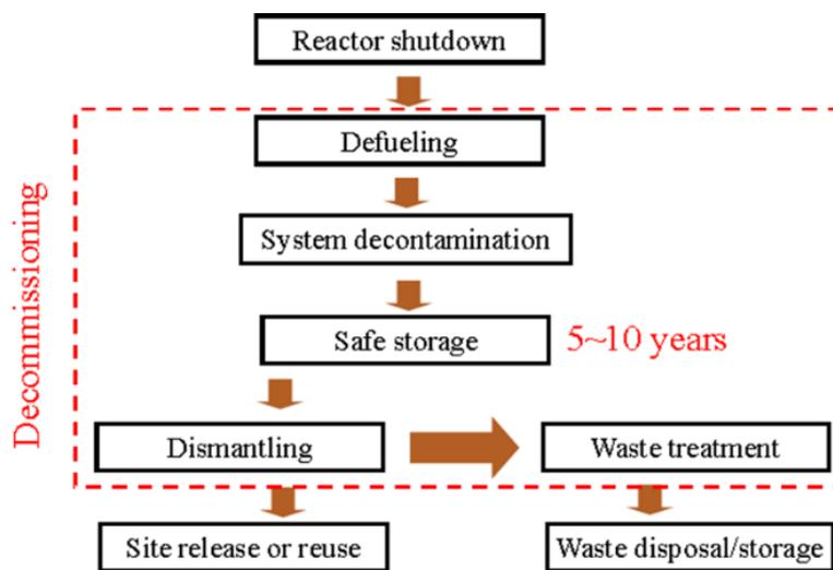
Figure 40 Example of nuclear power plant decommissioning process in Japan Information from the report of JAPCO and University of Fukui<sup>35</sup>. Figure by APERC.
