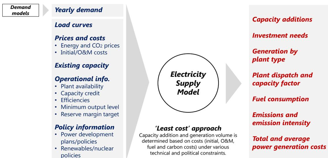
Figure 31 Electricity supply model structure
