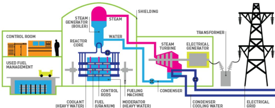
Figure 4 CANDU nuclear power reactor schematic diagram
