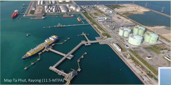
Today Thailand has completed LNG terminal which is operated by PTTLNG at Map Ta Phut and Ban Nong Faep, Rayong, with 11.5-MTPA and 7.5-MTPA gasification capacity, respectively.
