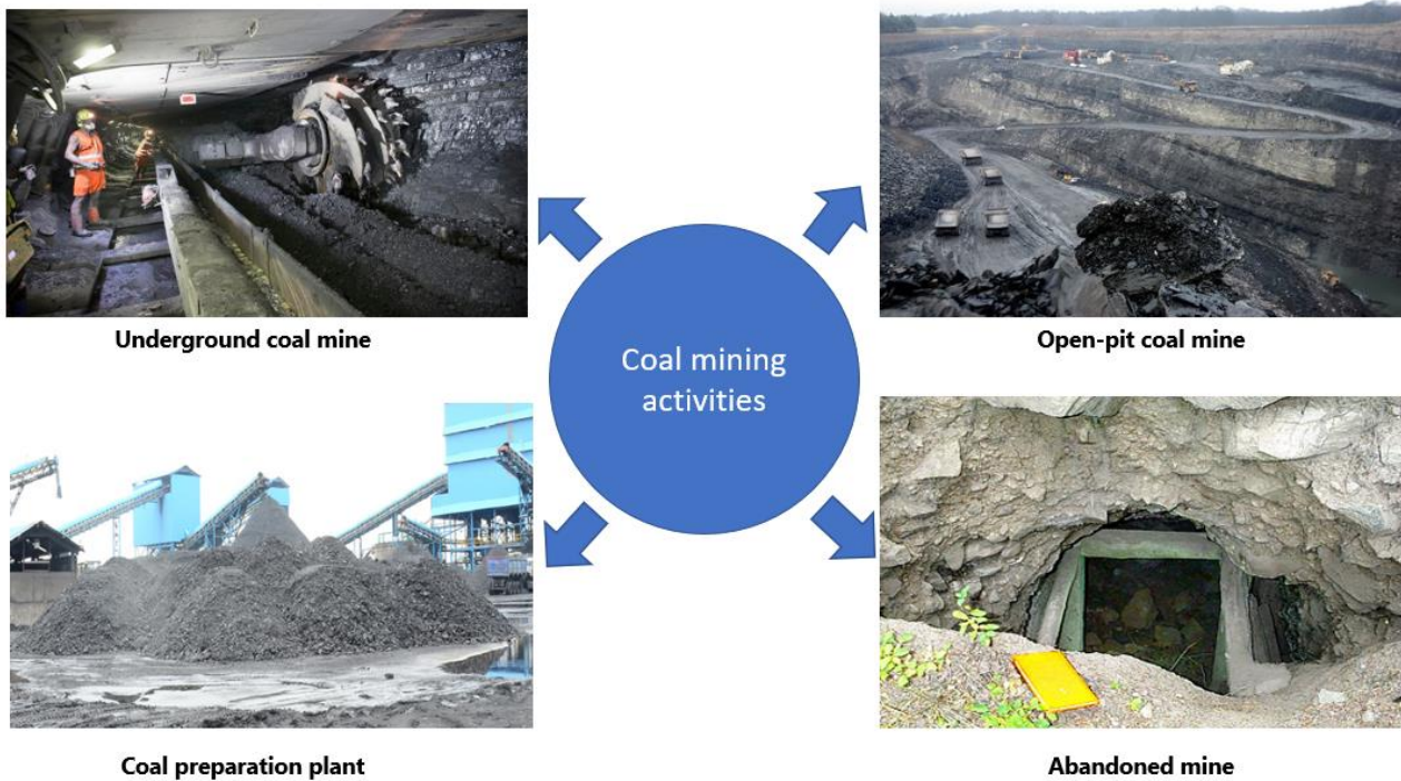
Figure 5.4: Sources of coal mine methane emissions
