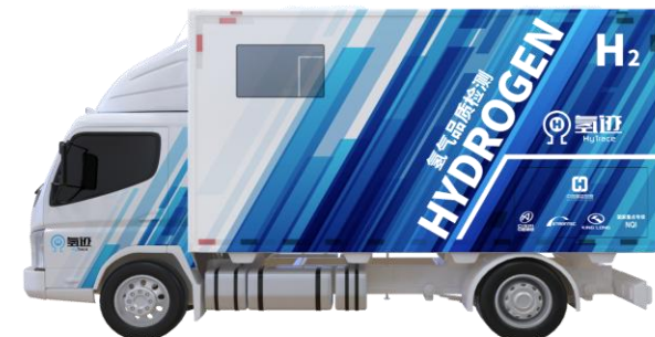
Mobile hydrogen quality testing vehicle
