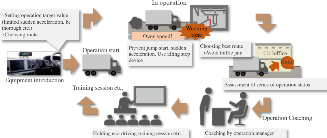
Figure 8 Image of Eco Driving Control System
